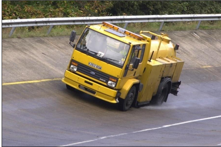
Figure 3.3 SCRIM testing a section of the TRL test track
