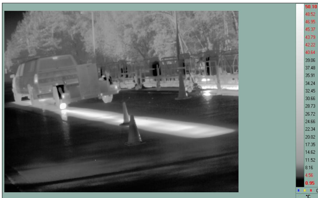
Figure 7.3 Thermal image of testing on a heated test section
