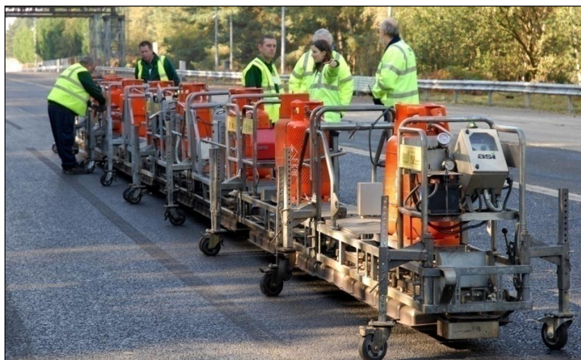
Figure 7.1 Heating rig used to heat the test sections
