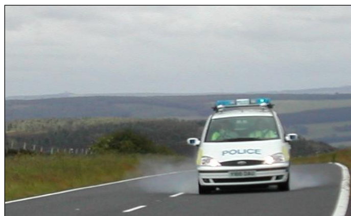
Figure 3.4 SkidMan equipped police car conducting a test
