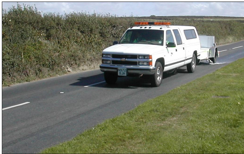
Figure 4.3 PFT conducting a wet test on the A389 trial site (Tyre marks in the nearside wheel path are due to previous dry testing)
